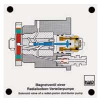
return flow with solenoid valve open
