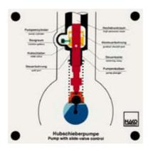
The end of injection is reached when the metering ramp reaches the gradual shut-off port in the slide valve.
