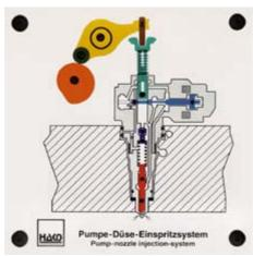
Function of the solenoid valve Pre-injection and main injection
