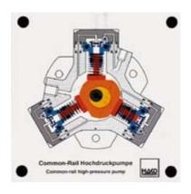
pump and the discharge of the fuel via the ball valve into a cellector line to the rail can be demonstrated.
