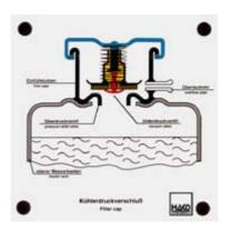
the pressure relief valve opens when the pressure gets too high
