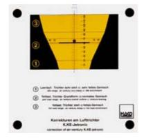
different openings of the air funnel, which depend on height of the opening and angle of the air funnel, can be read
