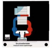
the gas column slide is moved along a curved path, so that the actual flow conditions can be shown
