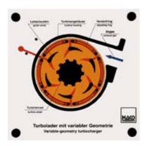
objective: torque increase in lower speed range
