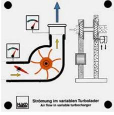
If the engine speed is too low, the cross-section is reduced, the output rotor turns more quickly
